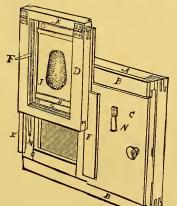
are grooved to receive the edges of the frame which carries the Vignetting card or design. By these devices the card-holding frame can be adjusted a greater or less distance from the negative, and the sliding-frame, D, may be shifted to any desired position.
