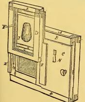
transversely over the slide. The inner surfaces of the frame, D, are grooved to receive the edges of the frame which carries the Vignetting card or design. By these devices the card-holding frame can be adjusted a greater or less distance from the negative, and the sliding-frame, D, may be shifted to any desired position.
