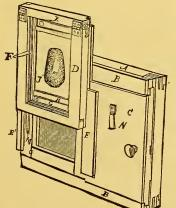
transversely over the slide. The inner surfaces of the frame, D, are grooved to receive the edges of the frame which carries the Vignetting card or design. By these devices the card-holding frame can be adjusted a greater or less distance from the negative, and the sliding-frame, D, may be shifted to any desired position.
